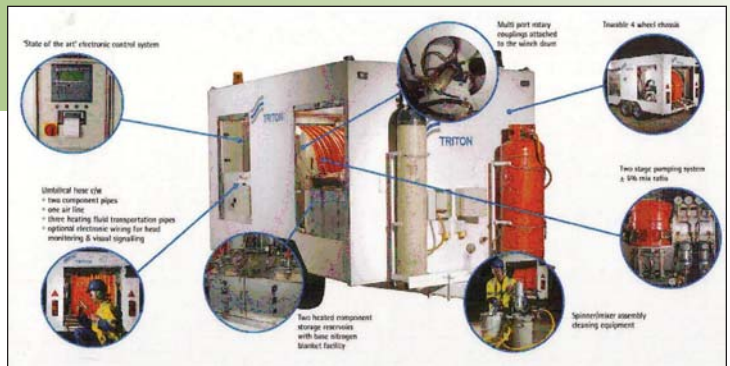
The lining process is undertaken using purpose built equipment. The equipment is designed to store, heat, pump, monitor, mix and spray polymeric formulations. The equipment and process has various stages, which when combined complete the lining process. The Lining Rig is powered by generator. The pumping system is air and hydraulic driven, the application head is powered by a 185 cfm compressor that is a separate unit.
