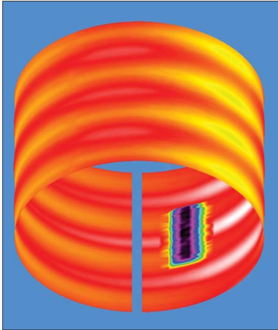
Figure 1 - Corrugated Polyethylene Pipe Data from a Prototype Profiler at the TTC.
